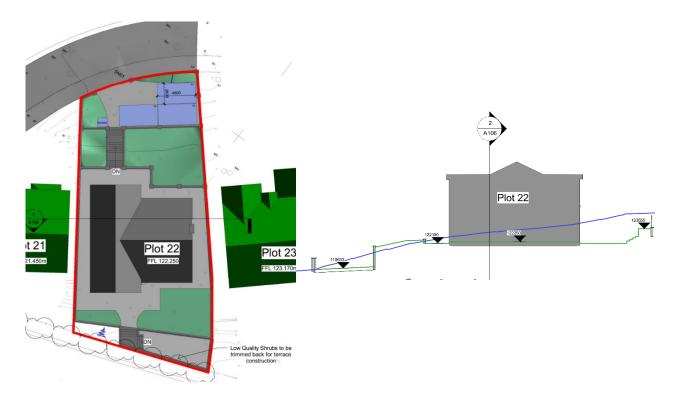
The amendments sought under this permission relate to the retention of the steps, which have been relocated from the centre of the site to the eastern boundary adjacent to Plot 23 (Number 4), the retention of the retaining wall and raised platform (amenity area) above, and changes to the front parking bay (including removal of front boundary wall).
